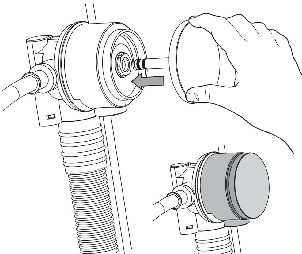
9, Fit the waste body and flange to the bath securing using screw and washer; ensure sealing washer is placed through the bath before this is done as shown on diagram. Use a pure Silicon sealant where necessary.
