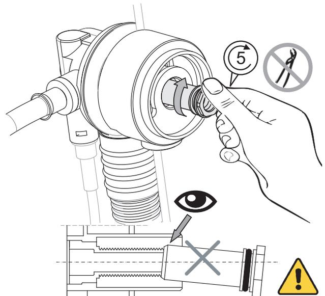
5, Tighten the nut to 4Nm
