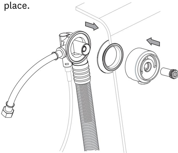
4, Turn the filter retaining nut clockwise, to secure in place.
