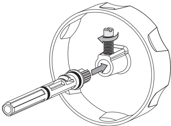
7, Place handle and fixing through the hole in overflow waste body.
