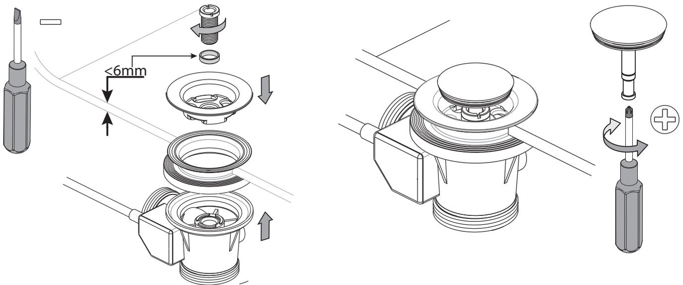
9, Cut any excess tube and fit into waste body using washer and nut provided.
