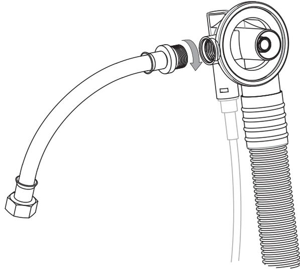
3, Fit the overflow waste body to the bath ensuring overflow washer is in place.
