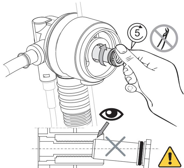
5, Tighten the nut to 4Nm
