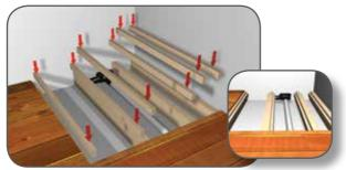
All exposed joists will now need a noggin or batten running along the inside of the joist to accommodate the new plywood low level floor. Measure the length of the exposed joist taking into account any obstructions. Cut some timber batten to length and screw at approximately 150mm intervals to the inside of all joists 18mm below the top of the joists.
