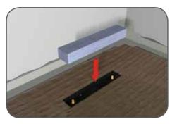
Step 23 Place the disposable tiling aid into the shower drain hole on the shower tray. The tiling aid provides the edge that needs to be tiled up to whilst protecting the drain from debris.
