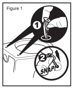
Insert the sprung retainers into the pan. Clip the tab - on the end of the wings - under the washer, before fitting through the WC and snapping into place with the hinge pillar bolt (Figure 1).
